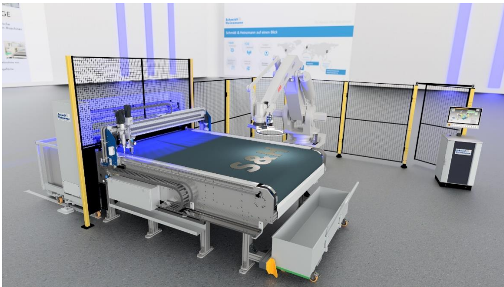
Camera system on cutting and stacking cell
