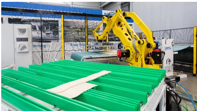
Press Automation including cutting unit “AutoCut”, scales with weight control and compensation function and robot handling.
